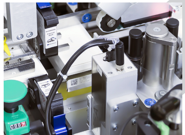
Thermal inkjet printing heads for 1D and 2D code and human readable data
