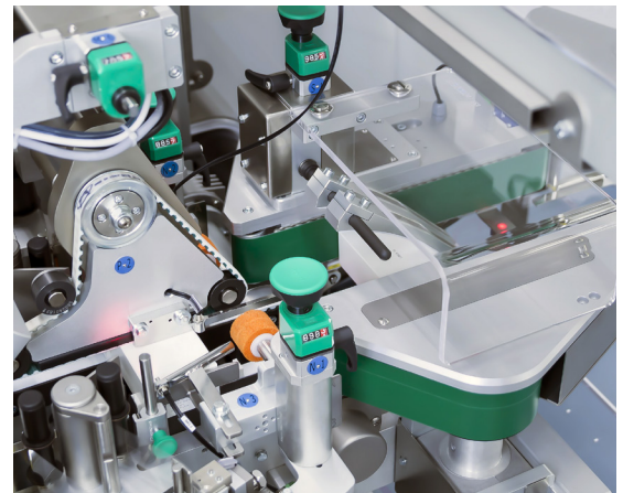
Carton reject by pneumatically driven flap
