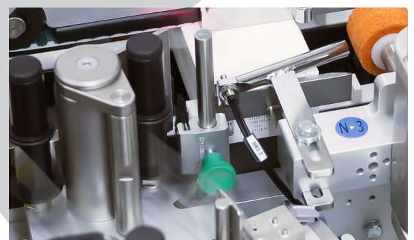
Tamper evident seal application on the closure point of folded carton
